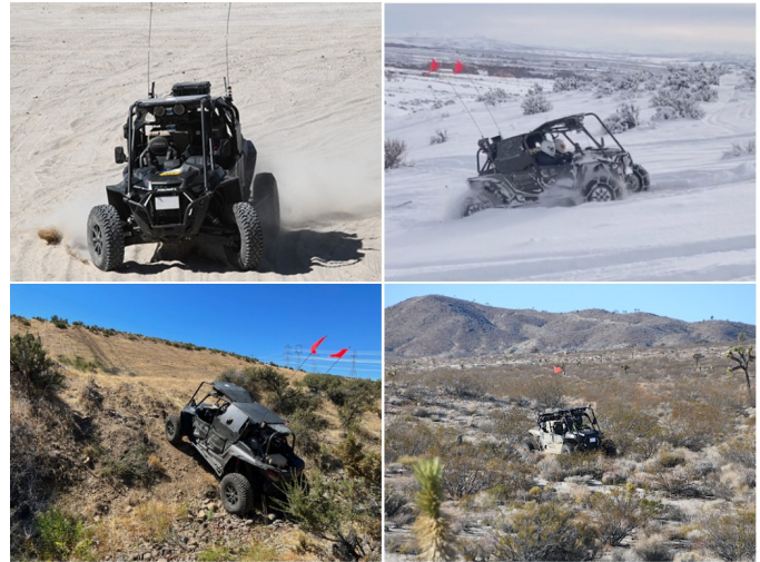
Fig. 1: High-speed driving in complex off-road environments requires joint reasoning of terrain semantics and geometry. Top row: a vehicle can drive at high-speed on a dirt road but has to be more cautious in snow due to wheel slipping. Bottom row: a vehicle needs to estimate terrain slopes and sizes of vegetation for safe planning and control.
