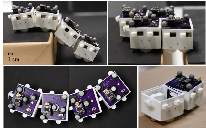
Fig. 1: Top: Robots can form a flexible chain and go down a step (left) or a rigid structure that crosses a gap between two equal-height test stages (right). Bottom left: Four robots forming an articulated chain. Bottom right: One robot inserts its anchor inside the opening of another one (circuitry removed for visual purposes).
