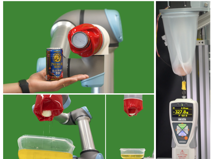
Fig. 1: From right to left, top to bottom: ROSE gripper on a robot arm picking a coffee can, and a peeled chicken egg submerged inside an olive oil container. The maximum lifting force that ROSE can endure is 328.7 N.
