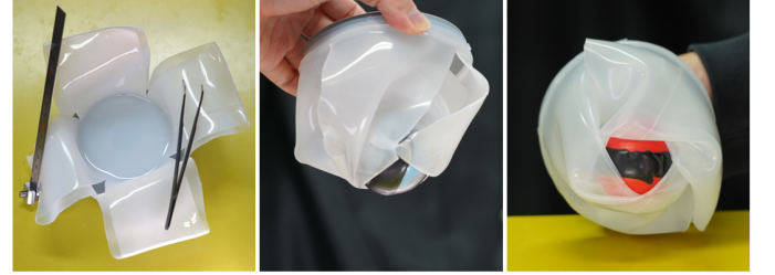
(c) Durability test result in case of critical damage (4 cut lines at 100% of skin height), from left to right: broken ROSE, front view, and bottom view of a broken ROSE successful grasping
