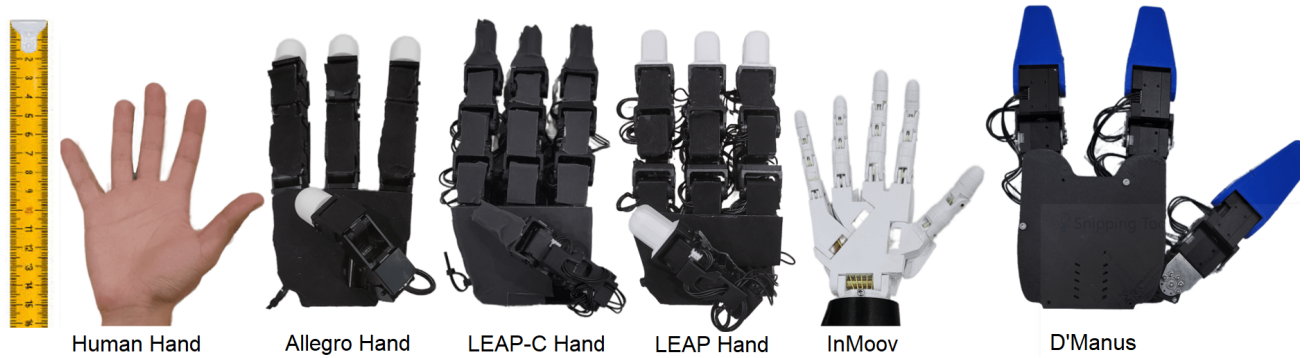
Fig. 3: Relative size of popular robot hands to scale. Left to right , adult human hand, Allegro Hand [20], LEAP-C Hand, LEAP Hand, Inmoov [18], D’Manus [21]. LEAP Hand is similar in size to Allegro and \sim 30\% larger than a human hand. D’Manus is considerably larger than the rest. Because of the tendon-driven nature, Inmoov is the smallest robotic hand. The hands are accurate to scale.
