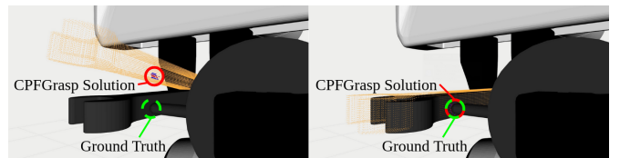
Fig. 3. Left: The CPFGrasp solution does not resolve the wrist wrench experienced by the robot. Right: The CPFGrasp solution is able to resolve the wrist wrench. \mathcal{L}_\Gamma allows us to distinguish between these cases.
