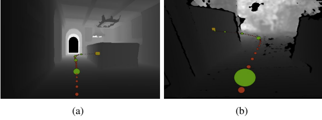
Fig. 5. Illustration of depth observation from simulation and the real world. (a) A depth image generated from the Gazebo simulation in the Matterport3D environment. (b) A depth observation obtained from Intel RealSense D435 during real-world experiments.
