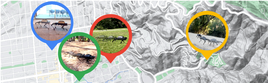
Fig. 1: We demonstrate that deep reinforcement learning can be used to efficiently train a quadruped robot directly on various real world terrains, e.g., flat ground (blue); soft, irregular mulch (green); grass (red); and a hiking trail (yellow), acquiring effective gaits within 20 minutes of training.
