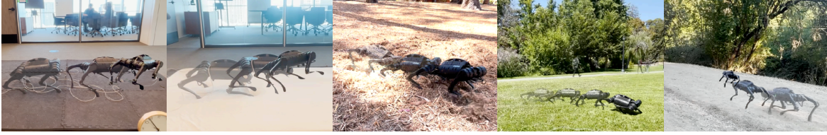
Fig. 2: Examples of learned gaits acquired on a variety of real-world terrains. Left to right: flat, solid ground covered in dense foam mats; a 5cm memory foam mattress; loose ground comprised of eucalyptus bark; a grassy lawn; a gently sloped hiking trail.
