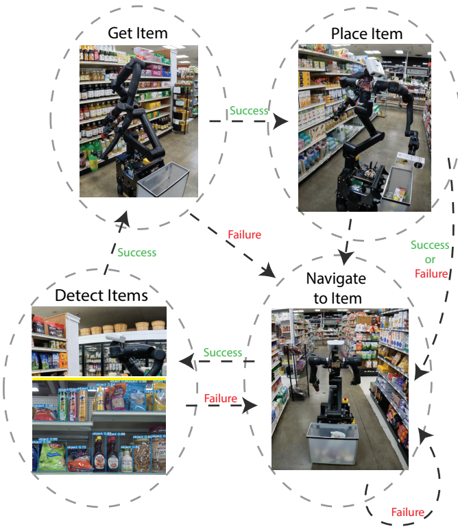
Fig. 5. Highly simplified task summary. Note that our hierarchical finite state machine includes many more states/transitions, but this provides a pictorial description of the main components of the grocery task.
