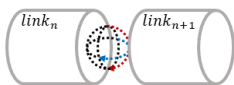
Fig. 5. There are two revolute joints between links, rotate along the x and y axis (blue and red).
