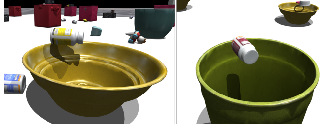
Fig. 9: Example of inaccurate simulation behavior in IG-CVXH due to a convex hull approximation of objects. The objects should fall into the bowls but are “floating” in the air because the bowls have been convexified
