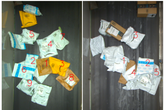
Fig. 4: Examples of ranking the packages based on the highest success probability estimate of their corresponding picks. A smaller rank number represents a higher priority.
