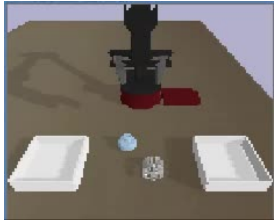
Fig. 11: Bin-Sorting task used for our simulated evaluations. The task requires sorting the cylinder into the left bin and the teapot into the right bin.
