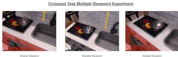
Fig. 17: Sample observations from different camera viewpoints, only used during fine-tuning. Left: the original camera viewpoint found in Figure 16. Middle: an elevated camera viewpoint where the robot and camera have been raised 7 cm. Right: a rotated camera viewpoint where the kitchen has been slightly translated and rotated 15 degrees counterclockwise relative to the camera and robot.
