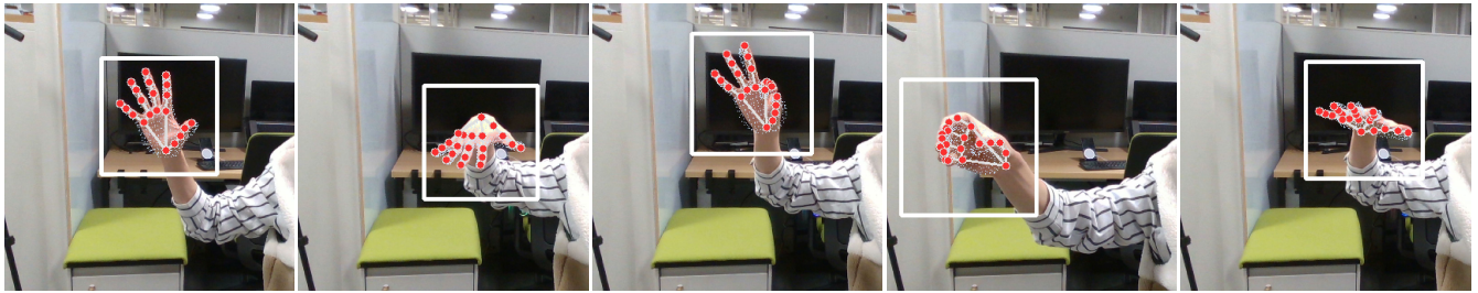
Fig. 7: Hand Pose Detection Visualization. This figure visualizes the hand detection results, with the white bounding box highlighting the predicted area and red points marking the identified finger key points. The hand skeleton is represented by the grey lines connecting the key points. Additionally, the small grey points depict the 2D projection of 3D vertices from the SMPL-X hand model. The figure showcases five diverse cases, from left to right: (i) a hand spreading out the fingers to initiate teleoperation, (ii) fingers facing downwards in preparation for a top-down grasp, (iii) a precision grasp using the thumb and index finger, (iv) a power grasp using all five fingers, and (v) a failure scenario where the hand is positioned vertically relative to the camera plane.
