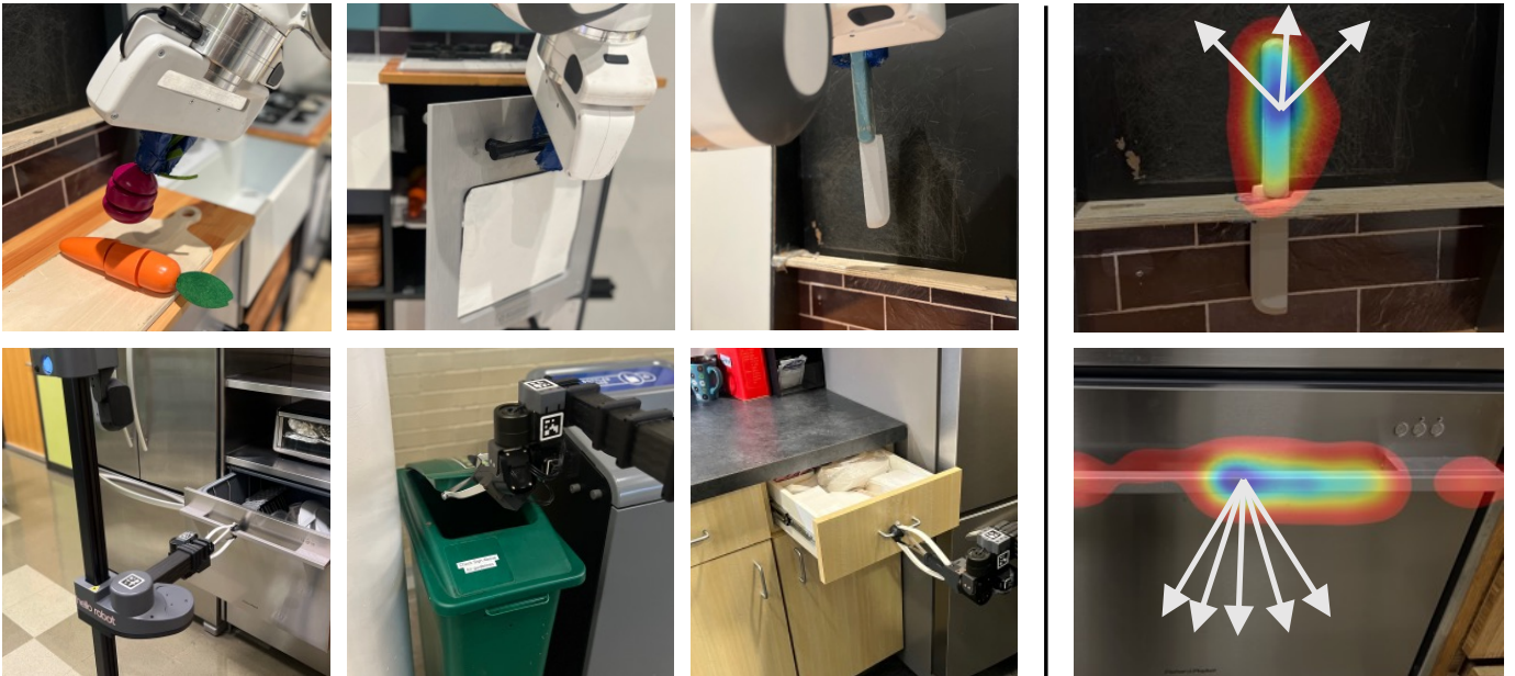
Fig. 4: We evaluate SWIM on six different real-world manipulation tasks on two different robot systems (shown on the left). On the right, we show a sample of the visual affordances from the visual affordance model \mathcal{G}_\psi
