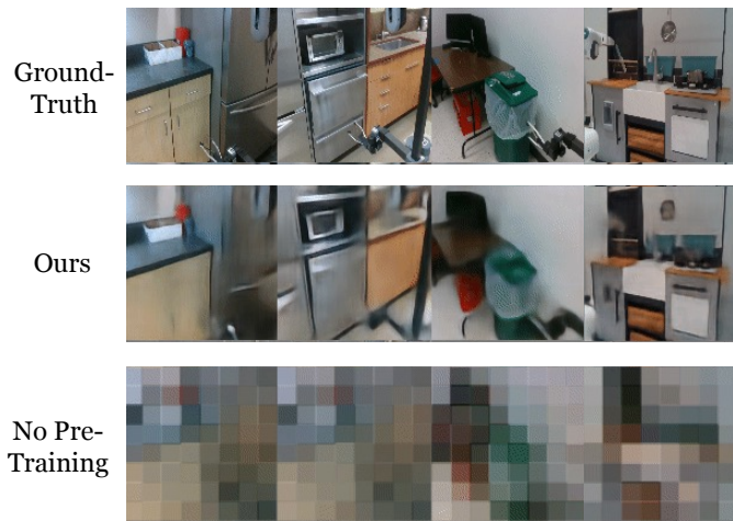
Fig. 8: Image reconstruction using world model features in early training stages for SWIM and MBRL-Affordance (which has no pre-training), showing that SWIM can effectively transfer representations from human videos. Note that for our experiments we use models trained to convergence.
