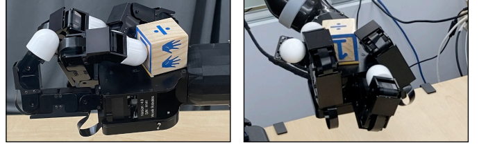
Fig. 9: Snapshots of the Allegro Hand while training an online policy using ROT. Here, we show that exploring along all action dimensions results in unsafe learning on the hand, driving it to undesirable positions and unnatural poses.
