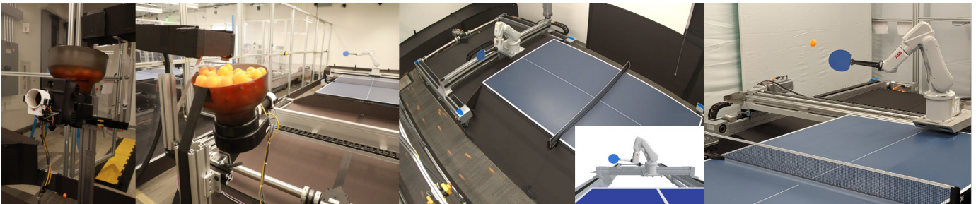
Fig. 1: The physical robotic table tennis system. Images from left to right show (I) ball thrower, (II) entire system (thrower, arm, gantry), (III) automatic ball refill, (inlay) simulator, and (IV) robot mid-swing.
