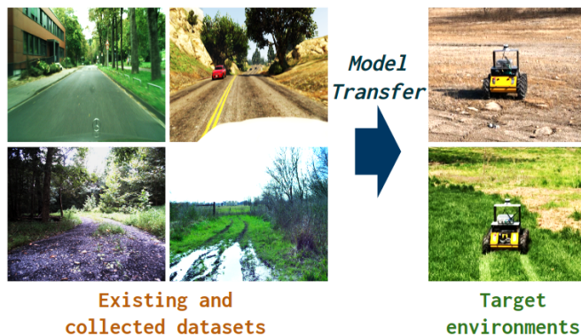
Fig. 1: Transferring models from the available domain to the target domain. The existing available data might be from either a simulator or collecting data in certain environments, at a certain time, and with certain sensors. In contrast, the target deployment might have significantly varying environments, time, and sensors.
