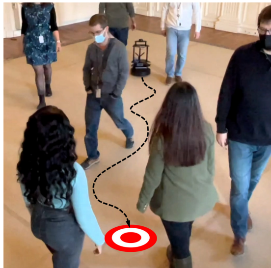
Fig. 1: The proposed DiPCAN architecture controls a robot (top) to reach a target location (bottom) while avoiding dense dynamic crowds using only the robot wheel odometry and narrow FOV depth camera. Videos of the experiments can be viewed at https://europe.naverlabs.com/research/dipcan .
