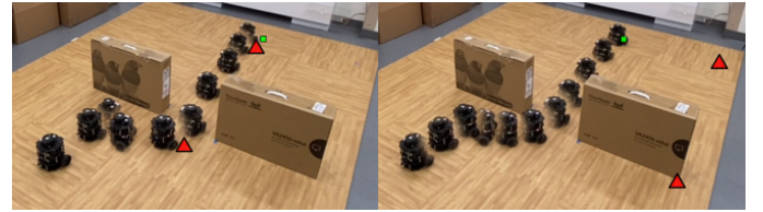
Fig. 5: Hardware performance of initial (left) and optimized (right) AGV designs. Square (green) shows the goal; triangles (red) show beacon locations. The optimized design eliminates drift relative to goal.
