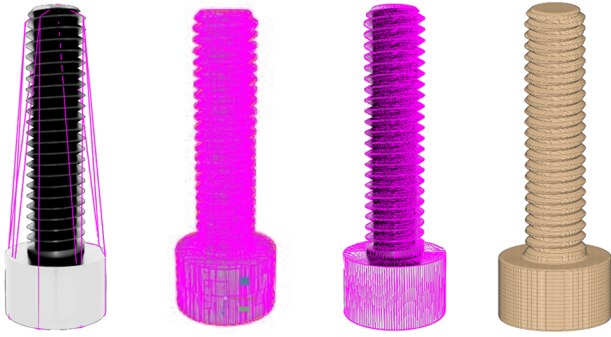
Fig. S10. Geometric representations, demonstrated on an M4 bolt. Left to right: Convex hull. Convex decomposition generated via V-HACD [64] (951 shapes). Triangle mesh representation generated in Onshape (47k triangles). SDF representation, visualized as a mesh of the isosurface.
