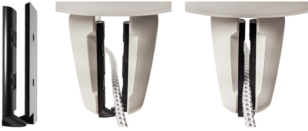
Fig. 4: Pinch-Cage (PC) Jaws . Left: a rendering of the design of the pinch-cage gripper jaws, which attach to the YuMi’s standard white gripper. Center: the cage grasp, in which the perpendicular “foot” segment of the attachment enables the cable to slide freely. Right: the pinch grasp, in which the cable is held tightly, preventing slack from slipping through.
