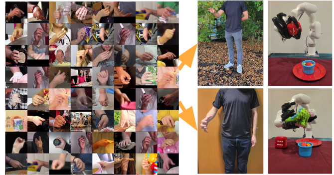
Figure 1: Our system leverages passive data from the internet to enable robotic real-time imitation in-the-wild. This low-cost system does not require any special gloves, mocap markers or even camera calibration and works from a single RGB camera.
