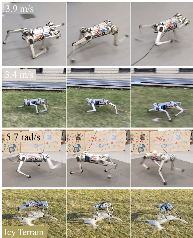
Fig. 1: An end-to-end learned controller enables the MIT Mini Cheetah to execute: (a) fast sprinting at 3.9 m/s (top); (b) a rough terrain 10-meter sprint at 3.4 m/s; (c) high-speed spinning indoors; and (d) robust spinning on an icy patch. All behaviors are realized by a single neural network that is trained in simulation and deployed zero-shot in the real world.
