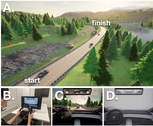
Fig. 8: CARLA Experiment Setup. (A) The stretch of highway that participants drove along. (B) Participants drove the simulated car using a steering wheel with accelerator and brake pedals. (C) and (D) show the difference in visibility in clear and foggy weather. Both cars are visible in the clear setting. In the fog setting, the car on the left is visible, but the car in the front can barely be seen.
