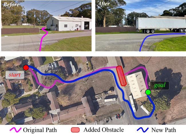
Fig. 10: On navigating with outdated hints, like the truck (top right) that is absent in the satellite image, ViKiNG uses its learned local controller to propose feasible subgoals that avoid obstacles and finds a new path (blue) to the goal that avoids the truck.
