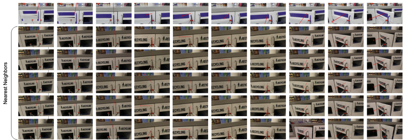
Fig. 10. The top row contains one rollout of VNN on a visually modified cabinet, under each image is the top 5 nearest neighbors from our demonstrations with the top one being the closest
