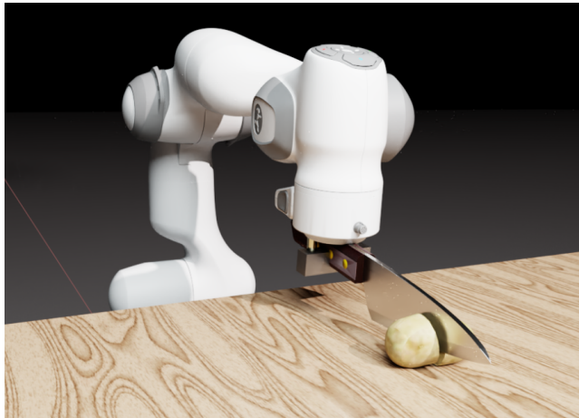
Fig. 1: A rendering from our differentiable cutting simulator. DiSECT provides accurate gradients of the cutting process, allowing us to efficiently fit model parameters to real-world measurements, and optimize cutting motions.
