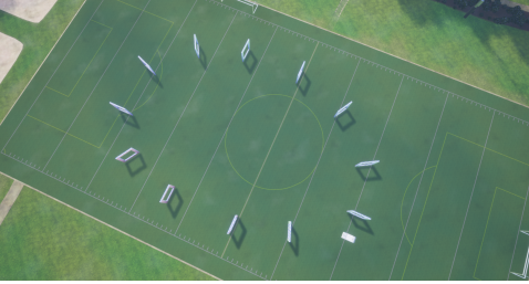
Fig. 8. Top view of Soccer Field Track in AirSim environment, where the HJB-RL policy is tested in simulation. At each oncoming gate, the HJB-RL policy is applied using the relative state of the quadrotor in a gate centered frame as input.
