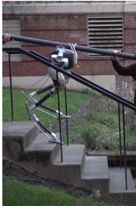
Fig. 3: The learned policies exhibit a high degree of blind robustness to a variety of stair-like terrain, and can reliably ascend and descend stairs of typical dimensions found in human environments.
