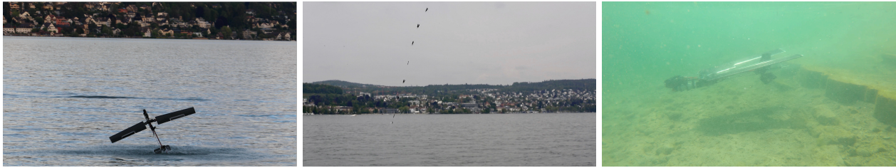
Fig. 1: Dipper platform in different configurations (from left to right): (i) emergence phase, (ii) sequential image during dive-in and (iii) underwater.
