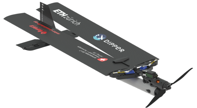
Fig. 10: Diving configuration with the wings and propeller folded backwards.
