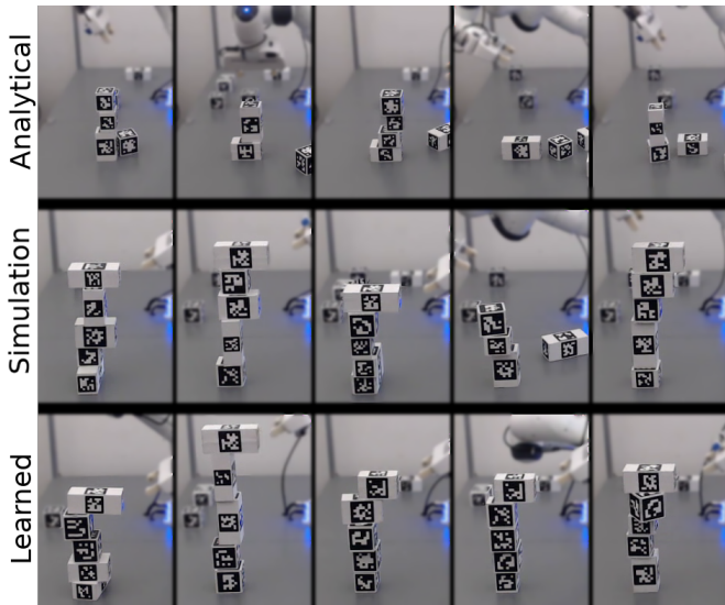
Fig. 7: Towers built for the Longest Overhang task when using different APF models. Observe that some towers built using the Analytical and Simulation models were unstable. See the appendix for more examples.
