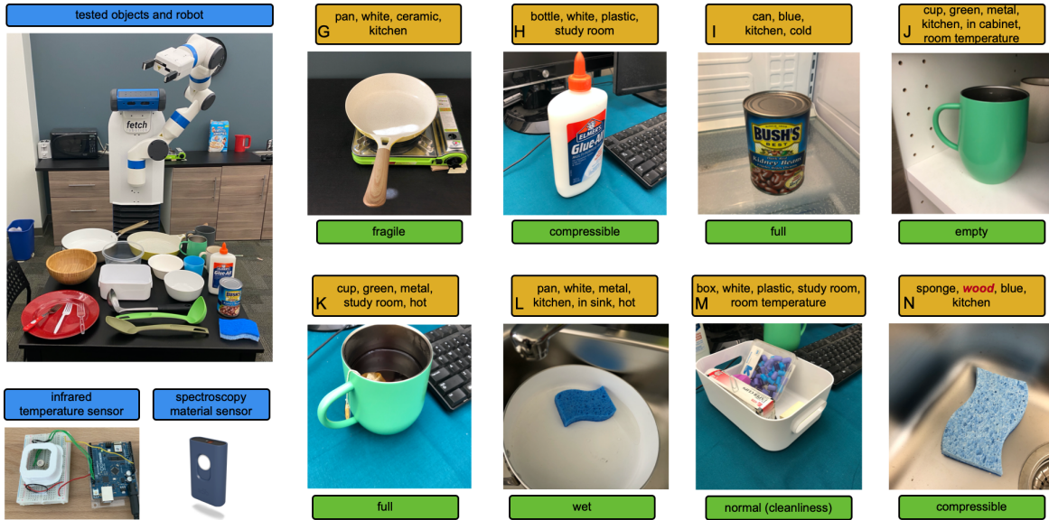
Fig. 9. The Fetch robot uses an infrared temperature sensor to detect the temperature and a spectrometer to detect the material of each novel object situated in different environmental contexts. Our model leverages extracted information (shown on top of each figure on the right) to predict an unknown object property (shown on bottom).
