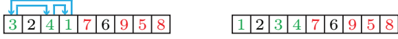
Fig. 2. [left] The initial configuration of an LOR instance with two cycles marked in different colors. A plan is shown that rearranges items following the cycle (341). [right] The resulting intermediate configuration.
