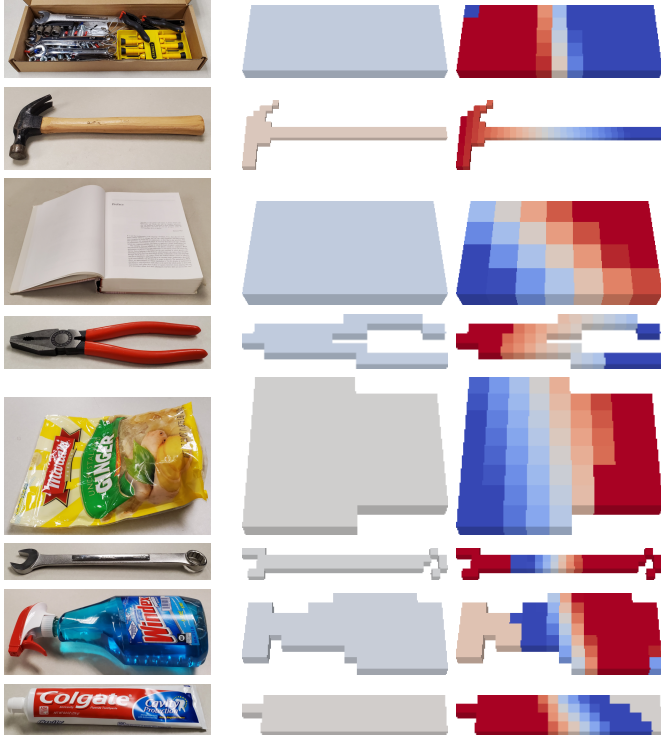
Fig. 3. Learned mass distributions. Red color means higher mass value while blue color means lower mass value. The middle column shows the initial uniform mass distributions provided to Algorithm 1 and the right column shows the mass distributions returned by the algorithm after only five iterations of gradient descent.
