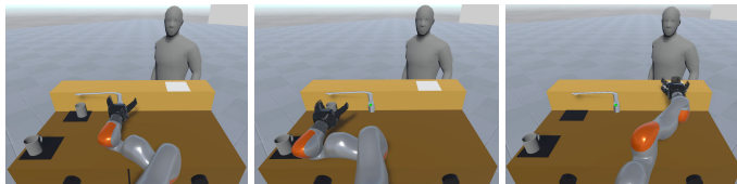
Fig. 1. Multi-stage manipulation: first fill the cup, then grasp it, and then deliver it. To avoid spills, a pose constraint is enforced after the cup is grasped.
