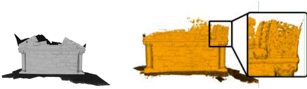
Fig. 5: Qualitative comparison of the model reconstructed by our approach at high resolutions on dataset D4: Left : Mesh provided by [29]; Right : proposed reconstruction with \alpha_{0,\lambda} = 0.1 cm. The zoomed-in view shows that the Level-0 model is able to retain minute texture details in the scene and create a high quality scene reconstruction using succinct Gaussian distributions as surface primitives.
