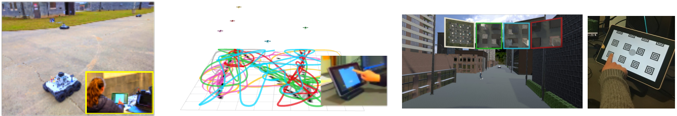
Fig. 1. Examples of our proposed method for user-based swarm control from user commands through the TanvasTouch Tablet interface. Here, we show results of dynamic swarm response to user-based inputs in (left) hardware experiments with a swarm of rovers conducted in real-world field testing environment, (middle) simulations with a swarm of quadrotors and (right) simulations of a swarm of drones providing visual feedback to a user in a Unity Virtual Reality game environment developed for end-to-end pipeline validation.
