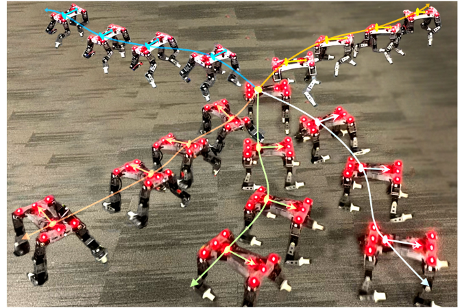
Fig. 1. A 12 degree of freedom quadruped (D’Kitty) discovers diverse locomotion skills without any rewards or demonstrations. We develop off-DADS, an asynchronous and off-policy version of Dynamics-Aware Discovery of Skills (DADS) [55], that enables sample-efficient skill discovery based on mutual-information based optimization.
