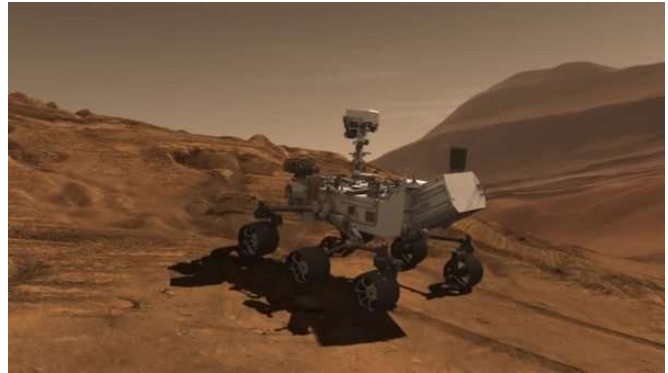
Fig. 1: In unstructured environments, the robot needs to make motion decisions in the navigable space with spatially varying terrestrial characteristics (hills, ridges, valleys, slopes). This is different from the simplified and structured environments where there are only two types of representations, i.e., either obstacle-occupied or obstacle-free. Evenly tessellating the complex terrain to create a discretized state space cannot effectively characterize the underlying value function used for computing the MDP solution. (Picture credit: NASA)
