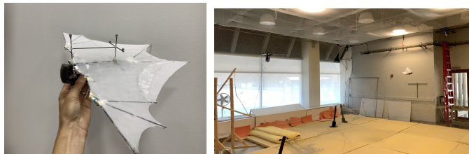
Fig. 1: Images of B2 (left) used in load cell and flight experiments and a free-flight experiment (right). The reflective markers are attached to the top carbon fiber structure in order to be elevated enough to minimize marker occlusions from the Vicon system.
