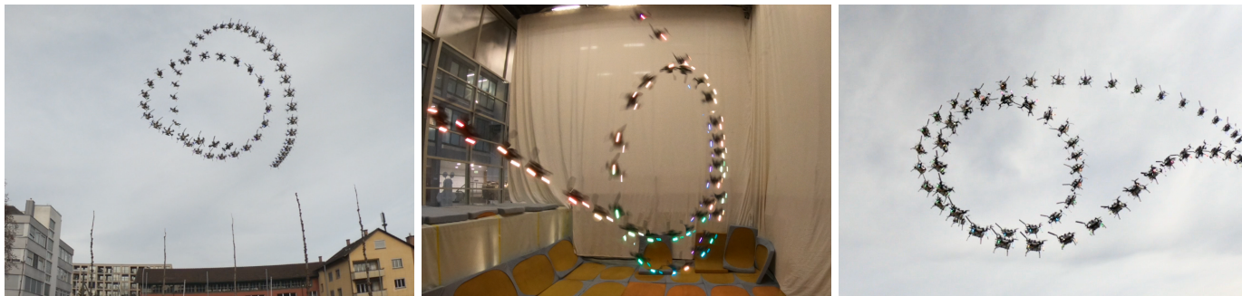
Fig. 1: A quadrotor performs a Barrel Roll (left), a Power Loop (middle), and a Matty Flip (right). We safely train acrobatic controllers in simulation and deploy them with no fine-tuning ( zero-shot transfer ) on physical quadrotors. The approach uses only onboard sensing and computation. No external motion tracking was used.
