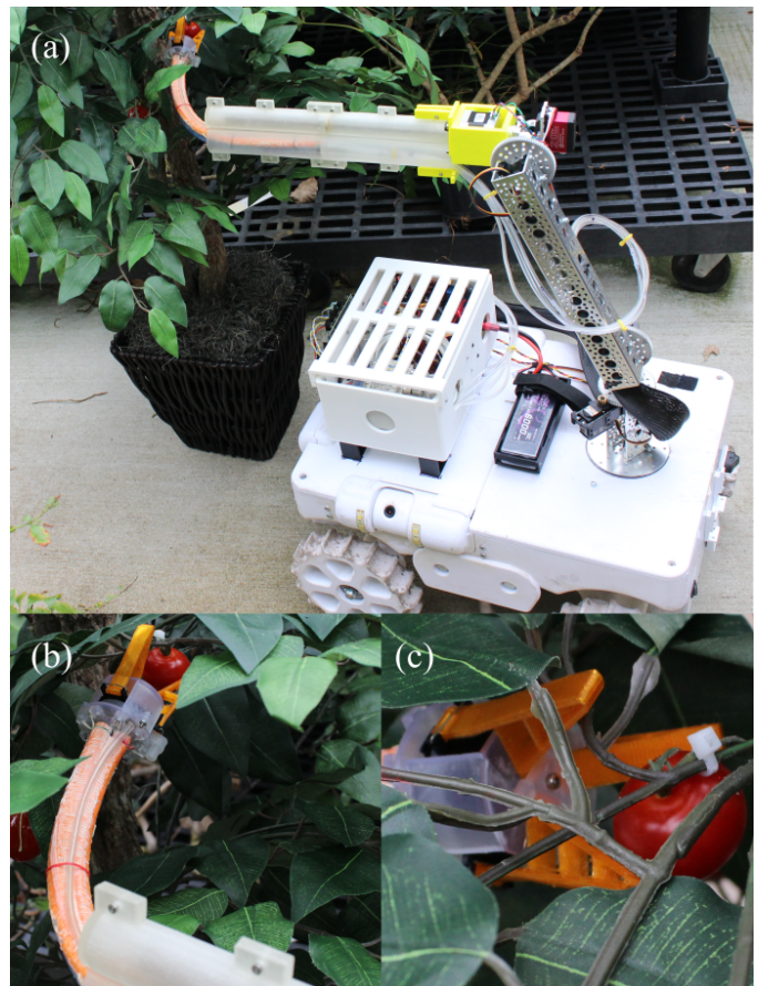
Fig. 1. (a) SoftAgbot system (mounted on a TerraSentia mobile rover) presented in this work picking a berry, (b) and (c) ability to reach bush interiors using a flexible soft continuum arm.
