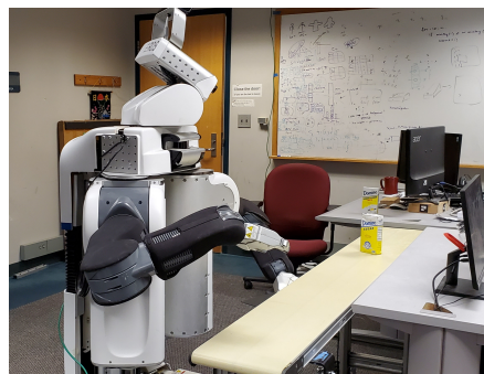
Fig. 1: A scene demonstrating the PR2 robot picking up a moving object (sugar box) off a conveyor belt.
