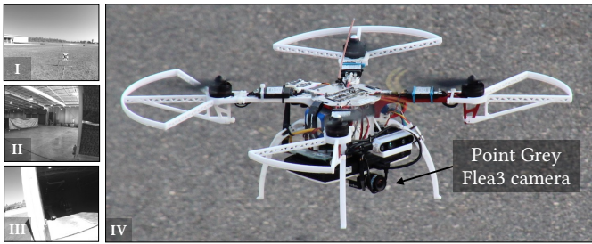
(a) MAV with a Point Grey Flea3 global shutter camera (IV) in three environments: outdoor (I), indoor (II) and transition (III).
