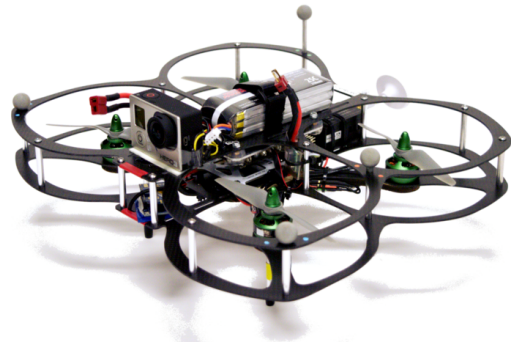
Fig. 5. The 750 g quadrotor used for the hardware experiments. Onboard computation is performed by an Odroid XU4 and the Pixhawk 1 Flight Controller.
