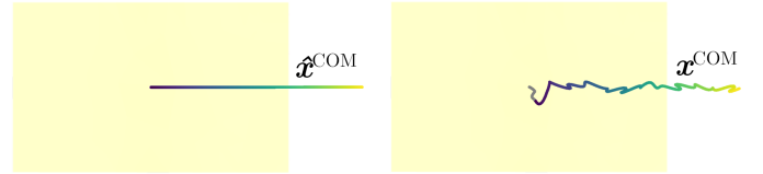
Figure 3. A top-down view of the Puppy 's target center of mass trajectory \hat{\mathbf{x}}^{\text{COM}} (left) for walking in a straight line, and the corresponding simulated center of mass trajectory \mathbf{x}^{\text{COM}} made with optimal control signals \mathbf{u} (right). In both cases the robot's body is shown at its starting position in yellow. Note that the short grey portion at the beginning of the simulated trajectory corresponds to the preparatory phase of motion, discussed in Section III-B.
