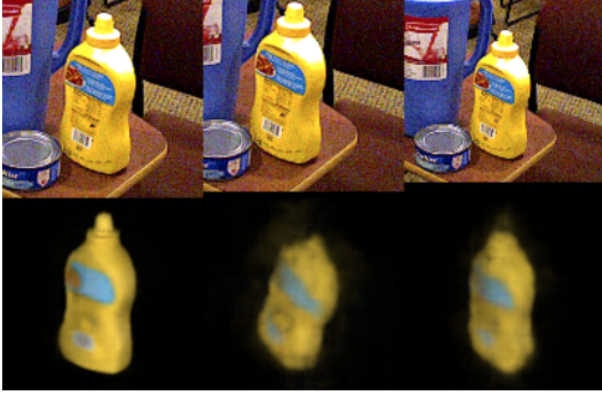
Fig. 4. Visualization of reconstruction of the RoIs from auto-encoder. Left is the groundtruth RoI. The other two column show the reconstruction with shifting and scale change. As it is shown the reconstruction quality degrades with deviations from groundtruth RoI. This property makes auto-encoder a suitable choice for computing the observation likelihoods.
