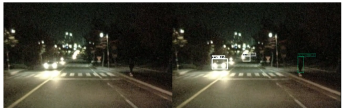
Fig. 3. Exemplary result from [1]. It has been shown that an RGB detector with temporary access to an infrared sensor can learn to recognize cars, persons, and objects at night in spite of the initial daytime only data.
