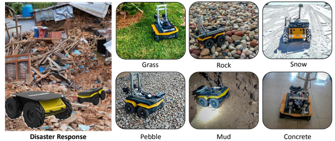
Figure 1. Motivating scenarios of robot adaptation to unstructured terrains. When mobile robots operate in a field environment during disaster response, the robots need the essential capability of navigating over a variety of terrains, such as grass, rock, snow, pebble, and mud, which often cannot be accurately structured before onsite robot deployment. In this paper, we propose the TRAL method to integrate representation learning and apprenticeship learning under a unified mathematical framework and estimate terrain feature importance to enable robust robot adaptation to unstructured terrains.
