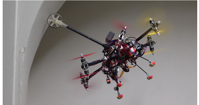
Fig. 1: Aerial manipulation platform in contact, rolling along a curved surface, with on-board state estimation.
